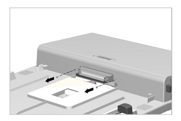
Figure 7-17. Removing the Computer Connector Screws
